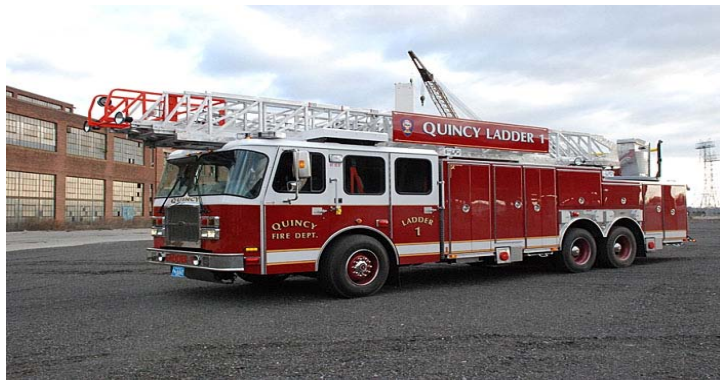
Quincy Ladder 1 2012 E-One 110 ft RMA, photo by M. Worley
