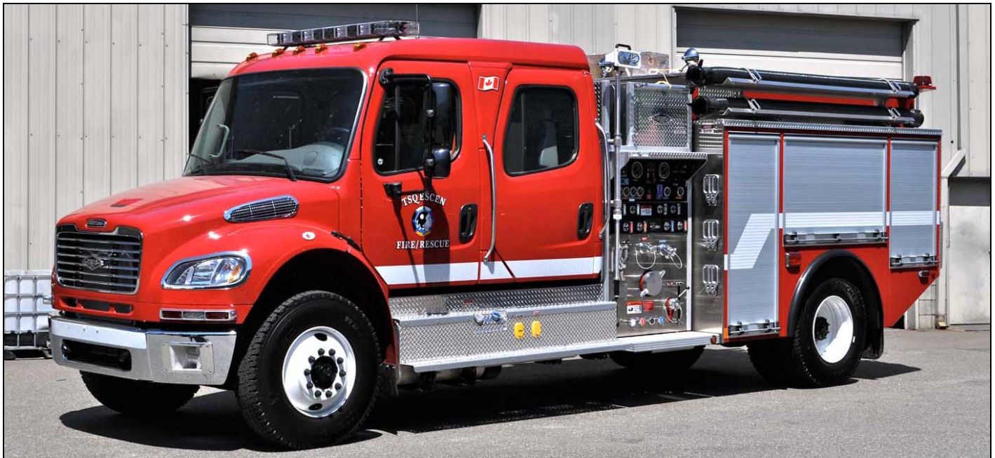
Tsq'escen FN in Canem Lake, BC received a 2012 Freightliner/Hub 840igpm, 500gwt, 25gft with a Foam Pro 1600 FS. New Westminster, BC Engine 3 is now running a 2011 Pierce Velocity PUC pumper with a 1250igpm pump, 400gwt and 40gft. It also has a Husky 12 foam system. SN 25135. (Terry Yip photos)
