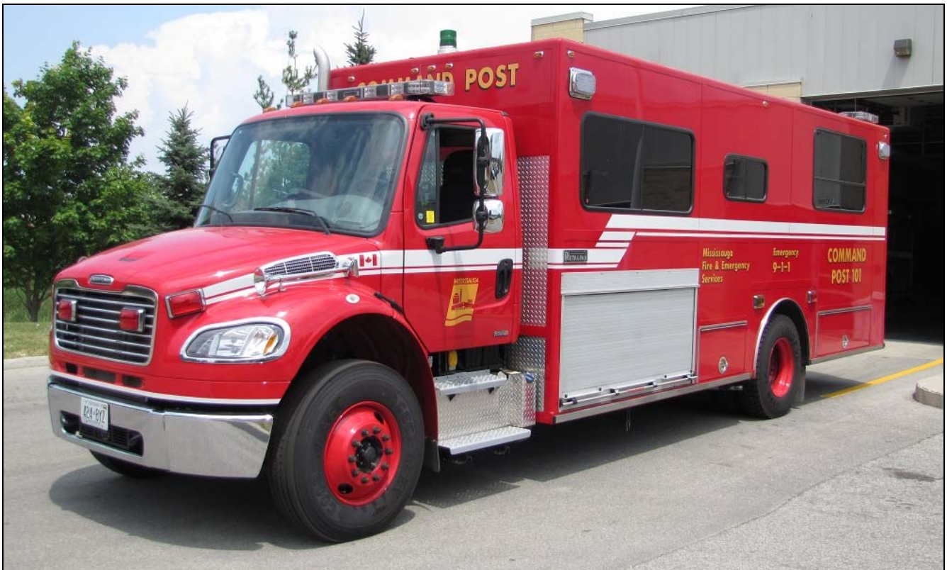
Command Post 101, remounted on a 2011 Freightliner M2 chassis by Peel Truck. The body is a 1997 Metalfab product. It is running from Station 117. (Desmond Brett photos)
