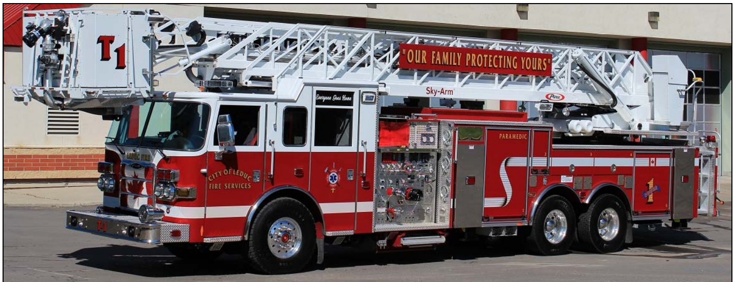
Leduc, AB's new Tower 1, a 2012 Pierce Arrow XT 1750igpm 250gwt, 20gft with a 100' Skyarm, (Dave Stewardson photo)
