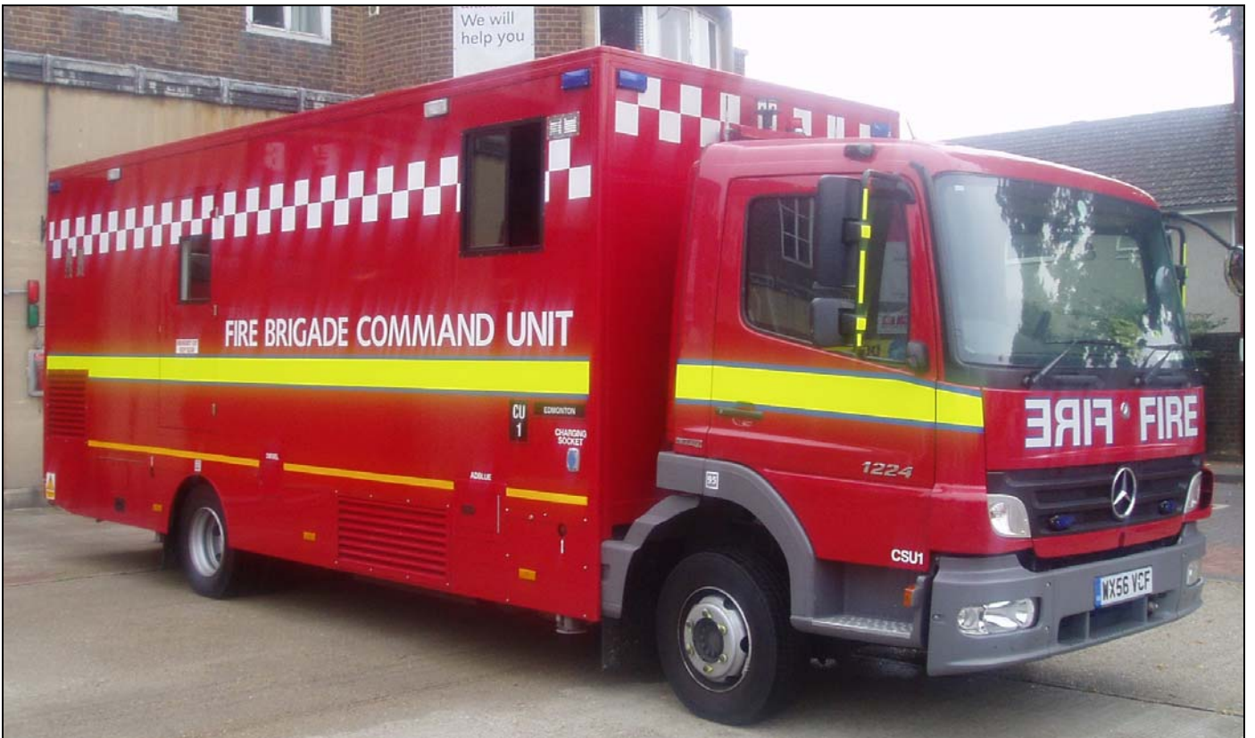
Command Support Unit 1, one of eight used by the brigade. Built on a 2006 Mercedes Atego 1224 chassis, it runs from A34, Edmonton. At major incidents, as many as four of these will be used.
