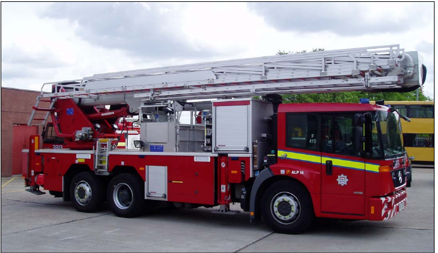
Above: One of the seven LFB Aerial Ladder Platforms (ALP 14). This 2007 Mercedes Eonic/Magirus runs from E41, Dagenham and has a 100' platform. (Bill Hickin)
