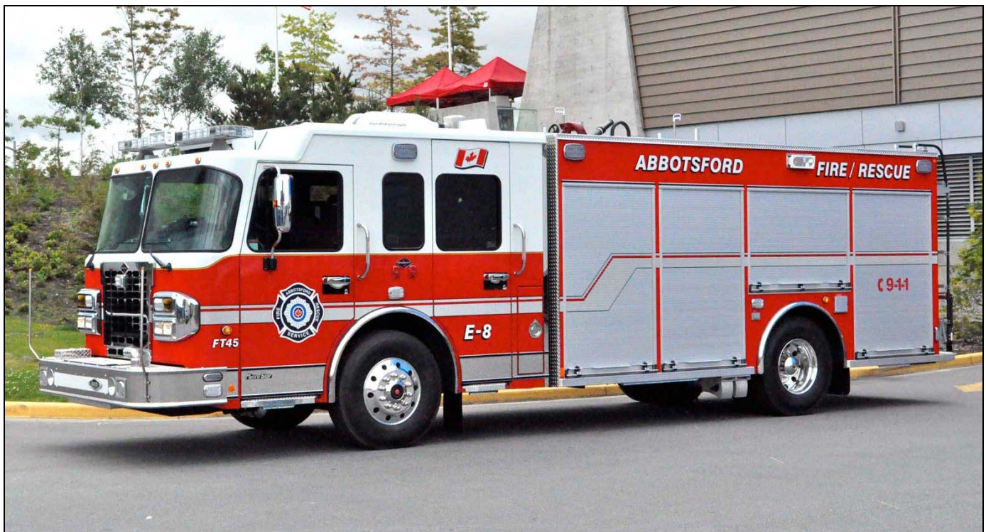
One of several new rigs now in service in Abbotsford, BC, Engine 8 is a 2012 Spartan Metro Star/Hub pumper with a 1750igpm pump and 500gwt. (Terry Yip photo)
