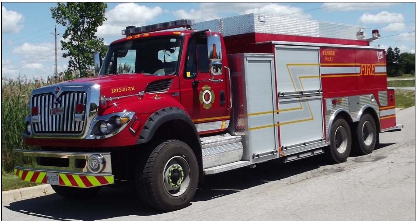
London's new tanker, assigned to Station 11, is a 2012 IHC/Carl Thibault 500gpm/2500gwt. (Rick Loiselle photo)
