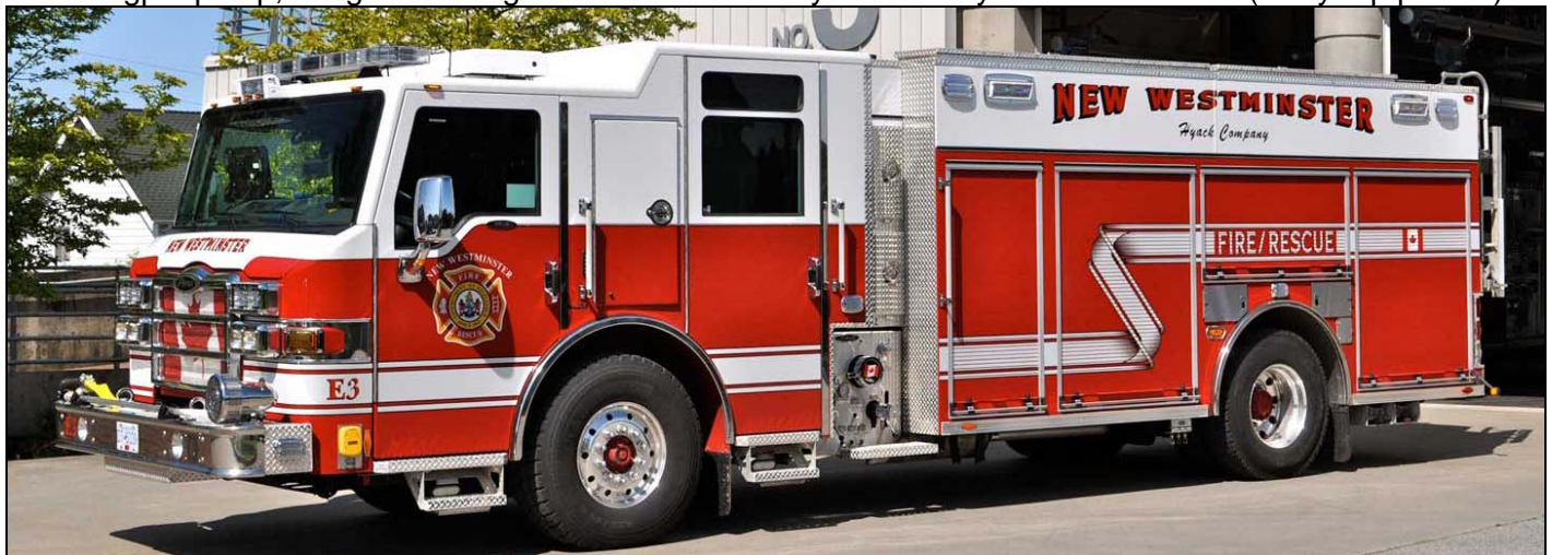
Tsq'escen FN in Canem Lake, BC received a 2012 Freightliner/Hub 840igpm, 500gwt, 25gft with a Foam Pro 1600 FS. New Westminster, BC Engine 3 is now running a 2011 Pierce Velocity PUC pumper with a 1250igpm pump, 400gwt and 40gft. It also has a Husky 12 foam system. SN 25135. (Terry Yip photos)
