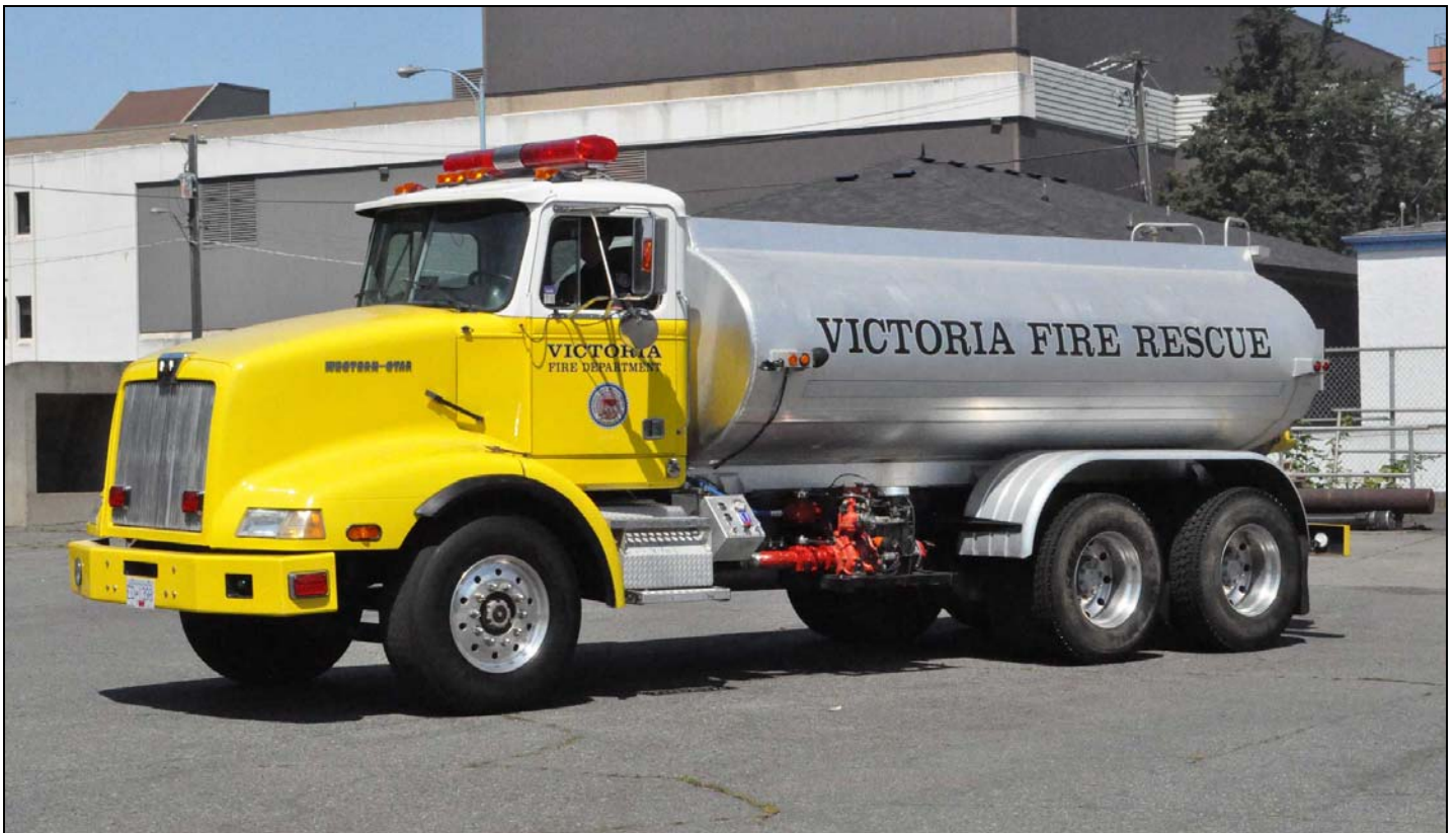
Also from the left coast, this Victoria, BC tanker is now occupying its third chassis. The 2500 gallon tank was originally attached to an old IHC streetwasher chassis, then was mounted on a Scot quint chassis when the ladder failed, combining it with a pump. This recent conversion has it looking pretty spiffy for a 1991 piece of equipment. (Terry Yip photo)
