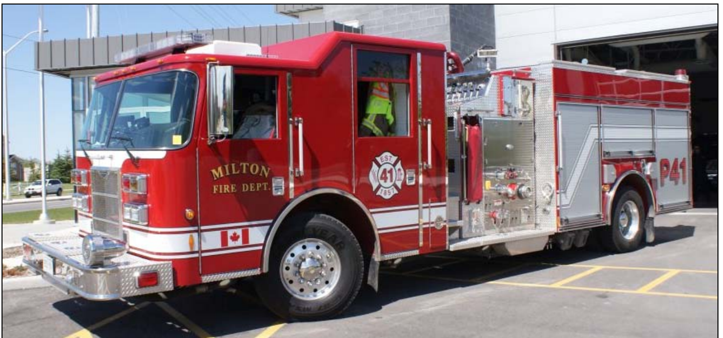
Milton, ON Pump 41 runs from Station 4 with a full-time crew. It is a 2010 Pierce Contender 1050igpm, 650gwt and 30gft. (SN#23365-1) (Ken Buchanan photo)
