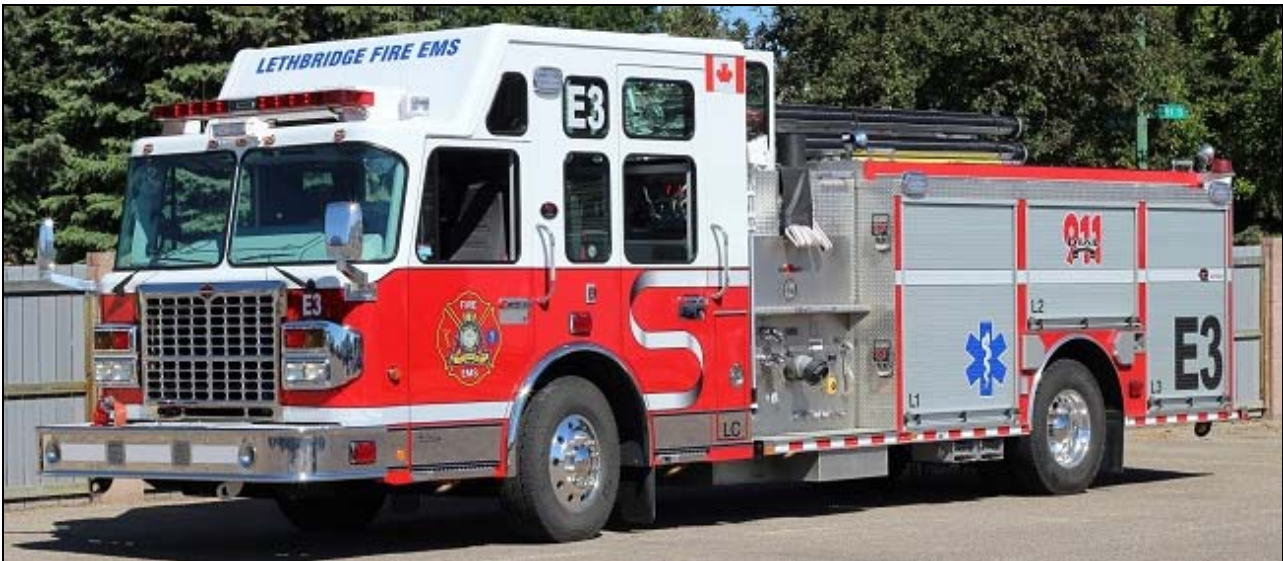
A new delivery for Lethbridge, AB. This 2012 Spartan Gladiator/Rosenbauer 1500igpm/550gwt/50gft is assigned to Engine 3. Below: Calgary HazMat 17, a 2009 Spartan/SVI. (John Bowerman photos).
