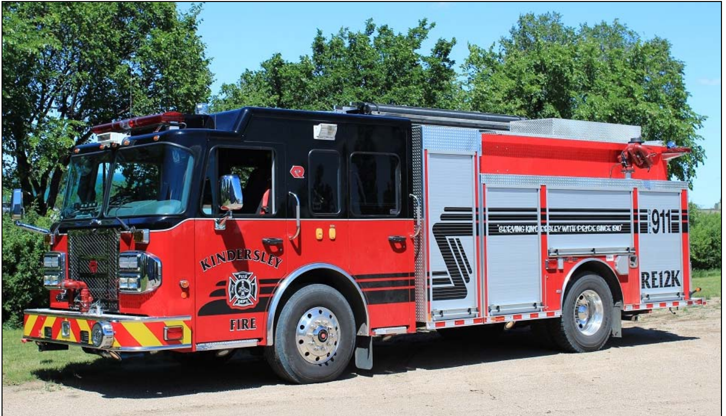
Rescue Engine 12K, Kindersley, SK's newest rig. This is a 2012 Spartan Metro Star/Rosenbauer 1050igpm/800gwt/30gft pumper. Below is Leduc, AB's new tower, a 2012 Pierce Arrow XT 1750igpm 250gwt, 20gft with a 100' Skyarm, (Dave Stewardson photos)
