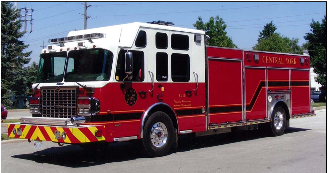
Central York Engine 411, another recent delivery, is a 2012 Spartan Gladiator/DEV 2000igpm/650gwt (SN CF211094). It runs from Headquarters in Newmarket. CYFS is replacing three more rigs this year, a pumper, a tanker and the platform. (Neil McCarten photo)
