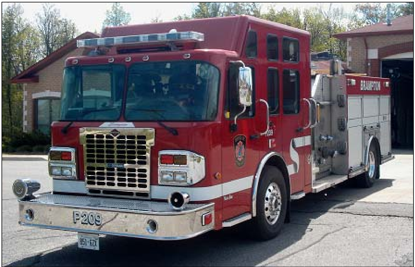
Two new rigs in service in the city above and slightly to the left of Toronto since our tour. P.209 is a 2011 Spartan Metro Star/Crimson/DEV pumper with a 1250igpm pump, 500gwt, 20gft and FoamPro 2002 FS. (Rob Simpson photo) A204 is a 2012 E-One Cyclone II 1750/250/20/95' tower. (Neil McCarten photo)
