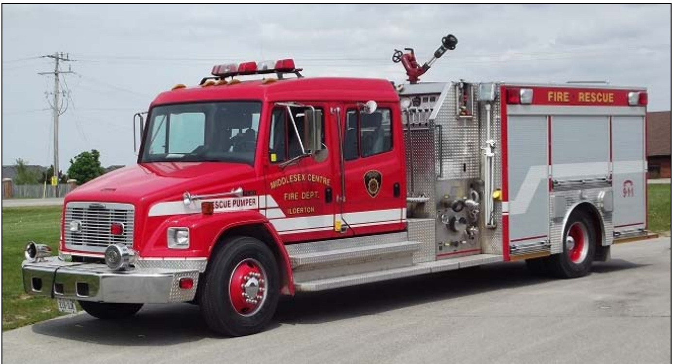
Another from the tour, this is Middlesex Centre RP1, a 2000 Freightliner/DEV 12050igpm/550gwt. It runs from Ilderton. (Rick Loiselle photo)
