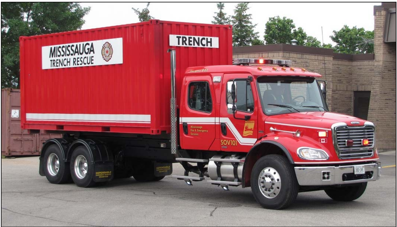
This is Special Operations Vehicle 101, inhabiting Station 114 when we visited (it alternates with H101 at Station 109). The truck is a 2006 Freightliner M2 equipped to handle pods, the Trench Rescue Pod was ordered at the same time.
