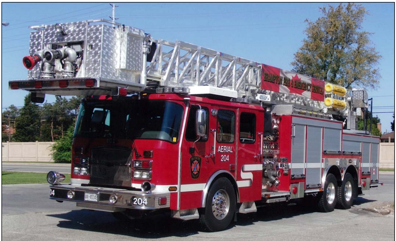
Two new rigs in service in the city above and slightly to the left of Toronto since our tour. P.209 is a 2011 Spartan Metro Star/Crimson/DEV pumper with a 1250igpm pump, 500gwt, 20gft and FoamPro 2002 FS. (Rob Simpson photo) A204 is a 2012 E-One Cyclone II 1750/250/20/95' tower. (Neil McCarten photo)
