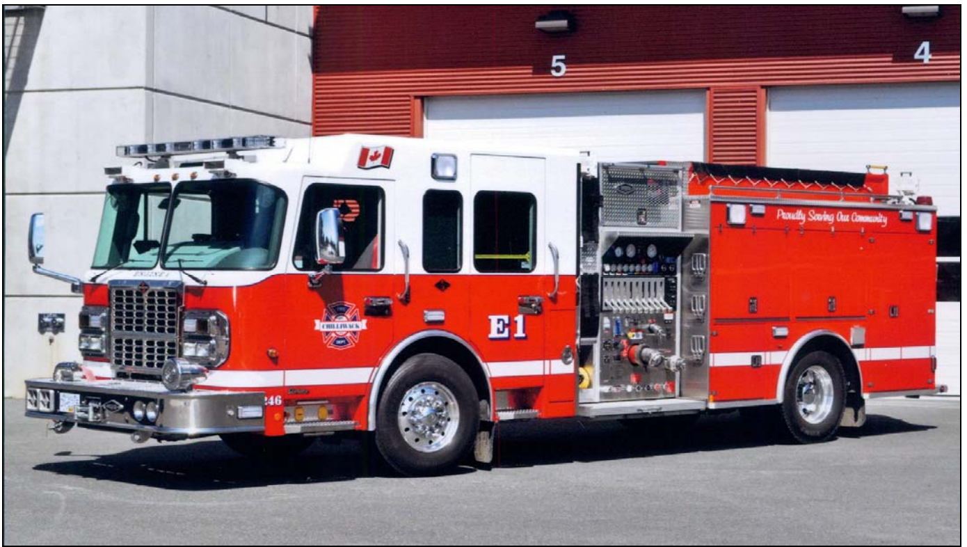
Chilliwack, BC now has two of these Spartan Gladiator/Hub pumpers. Engine 1, delivered last year, has a 1250igpm pump, 500gwt & 25ft, Engine 4 arrived last month, with a 1500gpm pump, 485gwt and 65' Snozzle . (Terry Yip photos)
