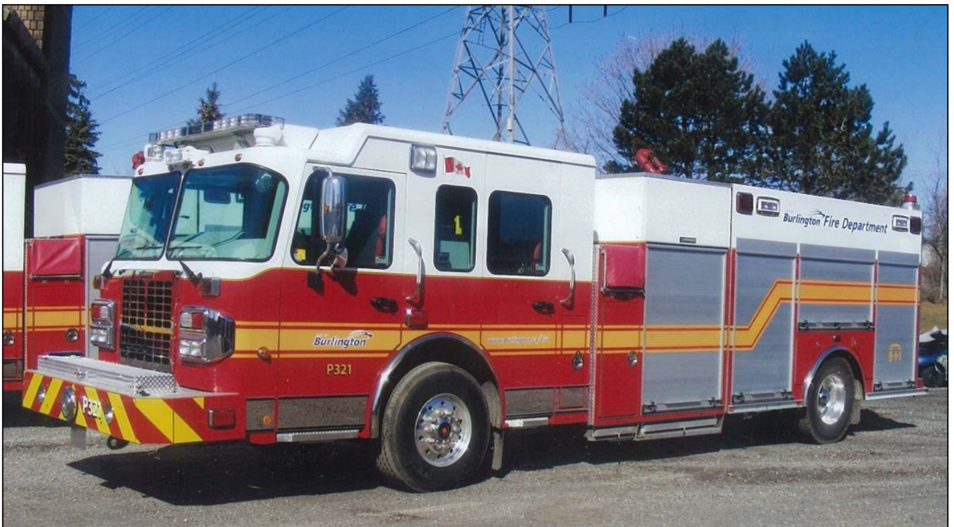
One of a pair delivered earlier this year, this is Burlington Pump 321, a 2011 Spartan Metro Star/DEV 1050gpm/500gwt/30gft. (Doug Holmes photos).
