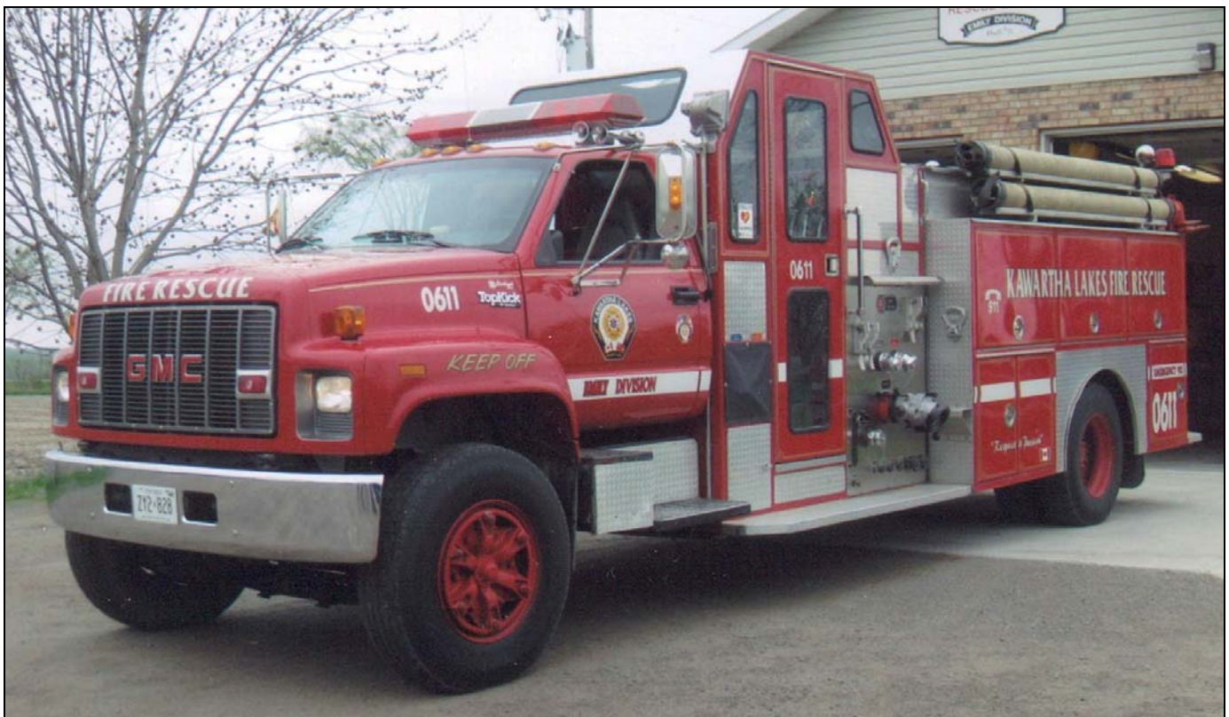
Seen on an OFBA tour, this is Kawartha Lakes Pump 0611, in Emily. This former township rig was built by Fort Garry on a 1995 GMC Top Kick chassis with 1050igpm pump and 900gwt. Unique units like this are fast disappearing from the KL roster as they standardize to Spartan chassis. (Larry Ward photo)
