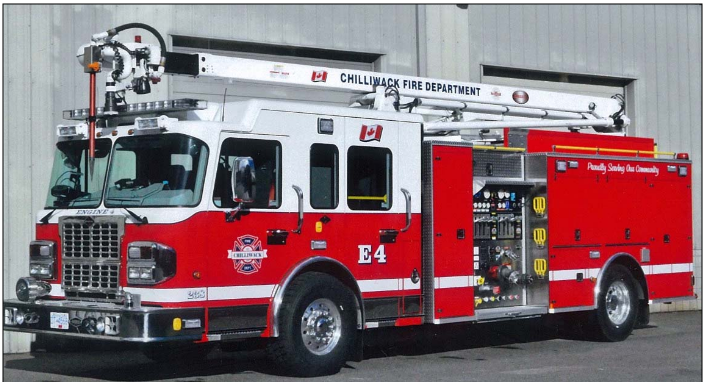
Chilliwack, BC now has two of these Spartan Gladiator/Hub pumpers. Engine 1, delivered last year, has a 1250igpm pump, 500gwt & 25ft, Engine 4 arrived last month, with a 1500gpm pump, 485gwt and 65' Snozzle . (Terry Yip photos)
