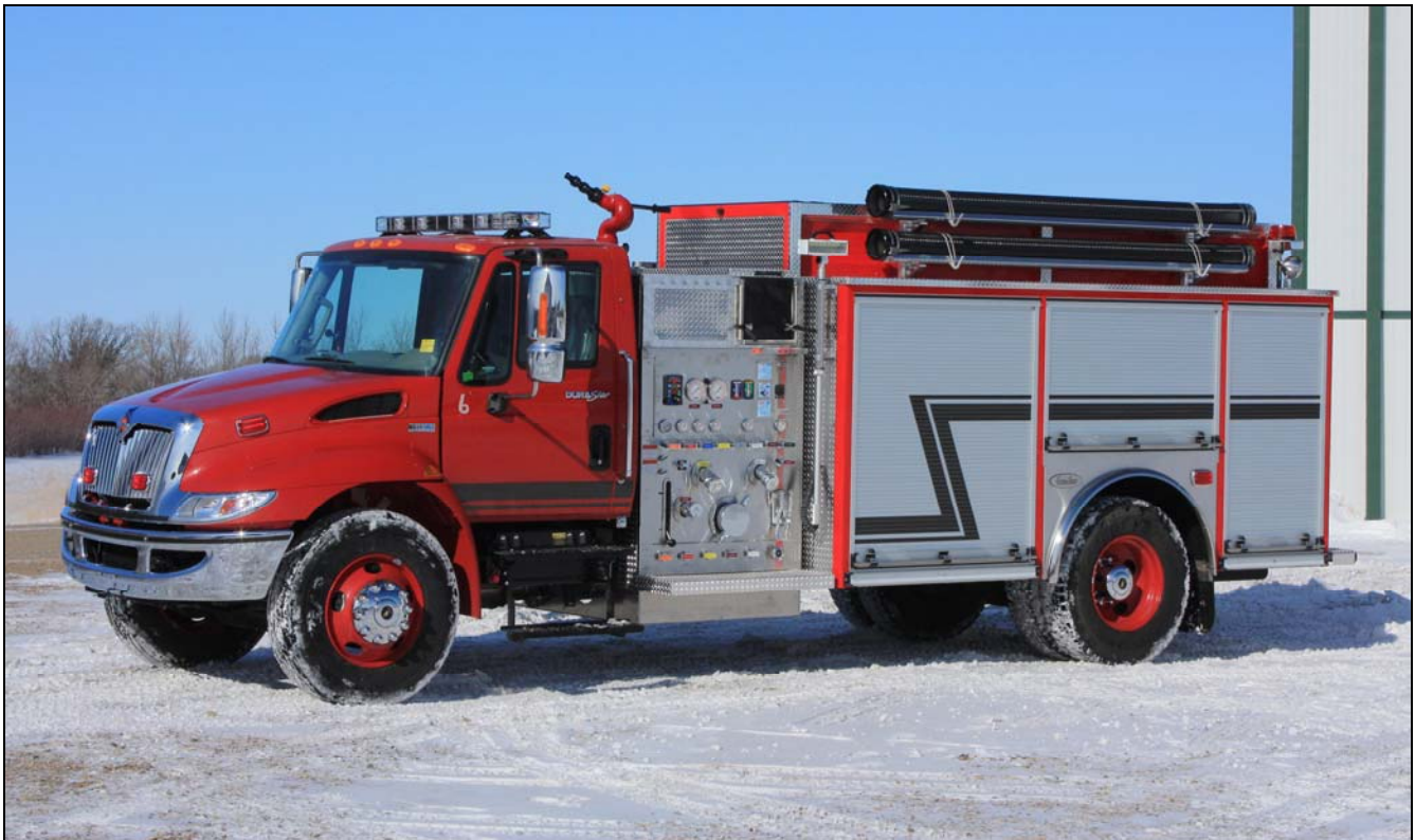
One of an order of six identical trucks delivered to first nations departments in Manitoba, this is a 2012 IHC 4300/Green Acres 840igpm/1000gwt. They were delivered to communities accessible only by ice road or air. (Dave Stewardson photo)
