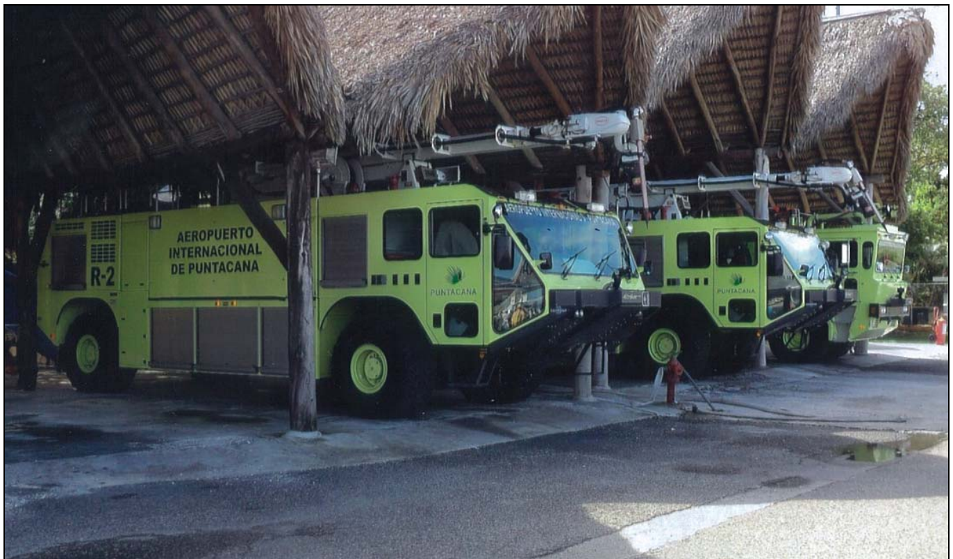
A pair of Osh Kosh Striker 1500s at Puntaacana Airport, in their unusual fire station. These Snozzle equipped crash trucks come with 2000gpm pumps, 1500gwts and 210gfts. (Doug Holmes photo).
