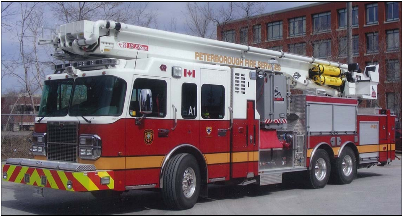
Peterborough just put this 2011 Rosenbauer T-Rex platform in service. Running from HQ, the rig is equipped with a 1250igpm pump, 300gwt, 30gft and a three-piece 115' tower.
