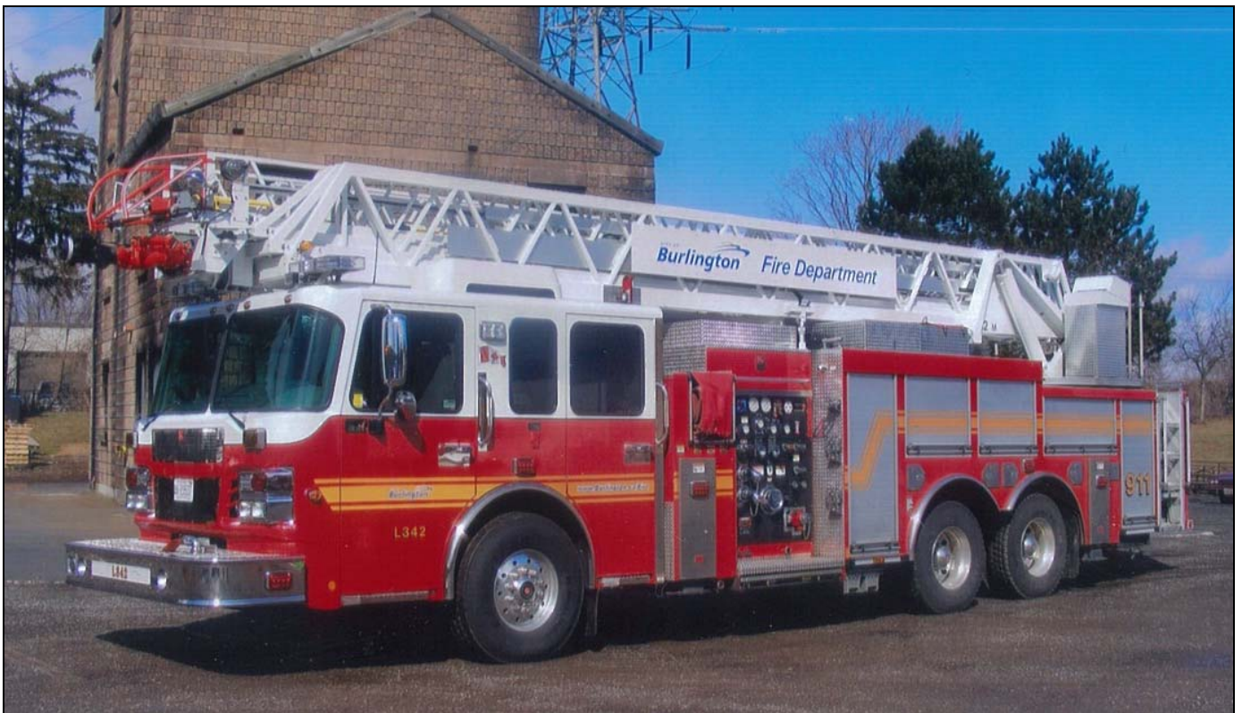
Burlington Ladder 342, a 2010 Spartan Sirius/Smeal 1050igpm/400gwt/20gft/105'.
