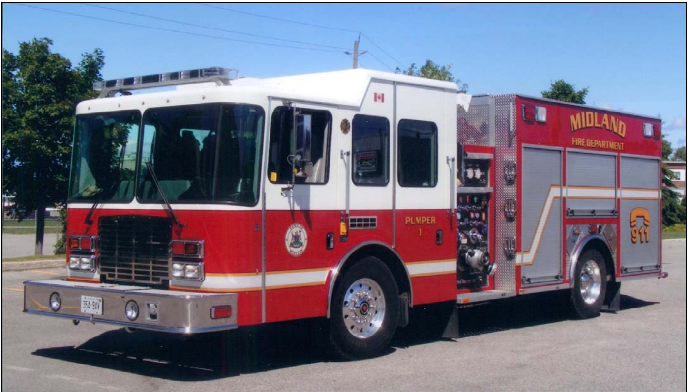
Midland Pumper 1, a 2010 HME/Ferrera with 1050igpm pump, 500gwt and 20gft.
