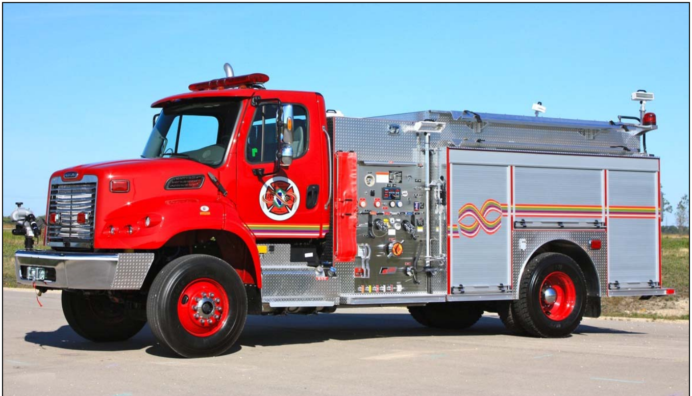
Fishing Lake Metis put this 2012 Freightliner M2/Fort Garry 840igpm/1000gwt pumper-tanker into service in October. Only the red cab and wheels are painted, the rest is chrome plated steel or aluminum. Based in Sputnikow, AB, it also has a Foam Pro 1600 FS. (Dave Stewardson photos).
