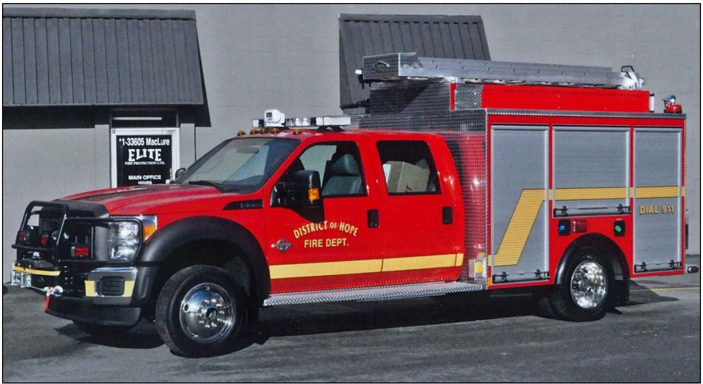
The District of Hope, BC recently took delivery of this 2012 Ford F550 4x4/Hub min-pumper. It has a 210igpm pump, 267gwt, 20gft and CAFS. It runs from Station 1. (Terry Yip photo).
