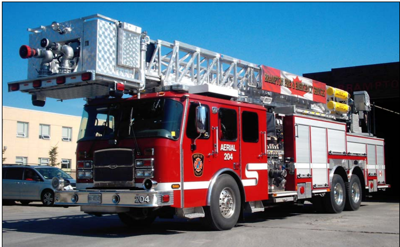
Brampton's newest acquisition is this 2011 Emergency One Cyclone II tower has a 2500gpm pump, 300gwt and 25gft. (Rob Simpson photo)
