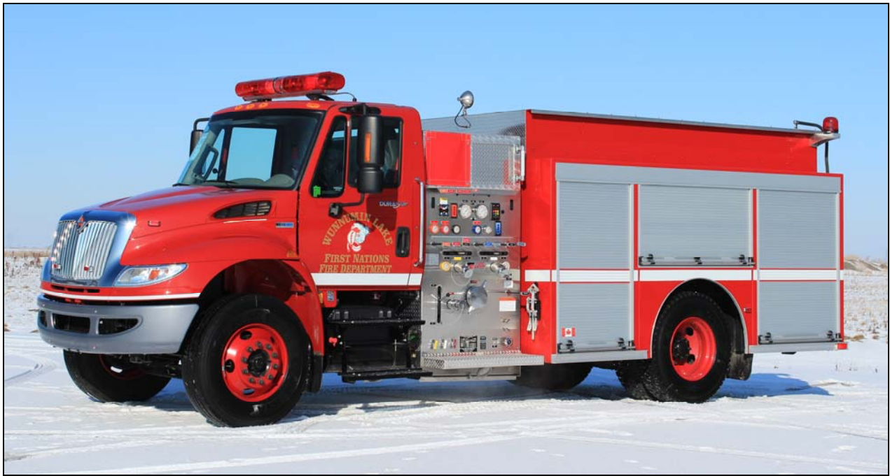
One of a number of trucks Fort Garry shipped via ice roads to Northern Ontario First Nations, this 1050/800/25 pumper was built on a 2012 IHC 4400 chassis, SN M303. It was delivered to the Wunnumin Lake First Nation. (Dave Stewardson photo)
