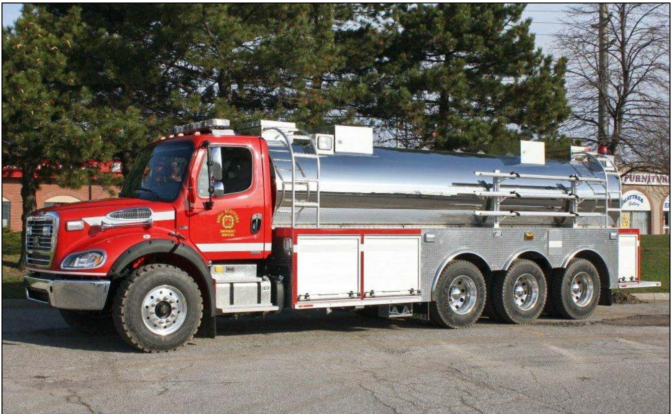
An even bigger industrial rig, this red and chrome one belongs to the Shell Refinery in Scotford, AB. Built on a 2011 Freightliner M2 chassis by Dependable, this is a 4000g foam tanker with a 468gpm pump, it was delivered last spring. (Bill Fairhurst photo)
