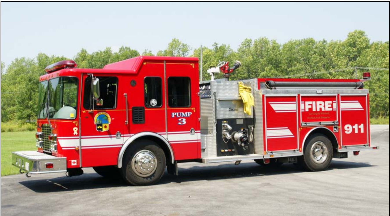
This 2002 HME 1871/Central States apparatus runs as Fort Erie Pump 3. It has a 1050igpm pump and 700gwt. (Jon Lasiuk photo)
