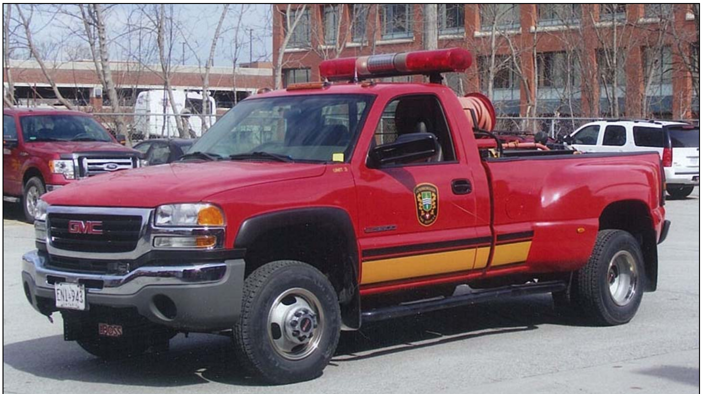
Peterborough Unit 3, a 2005 GMC 3500 4x4 chassis equipped with a portable pump and 200gwt. (Neil McCarten photos)
