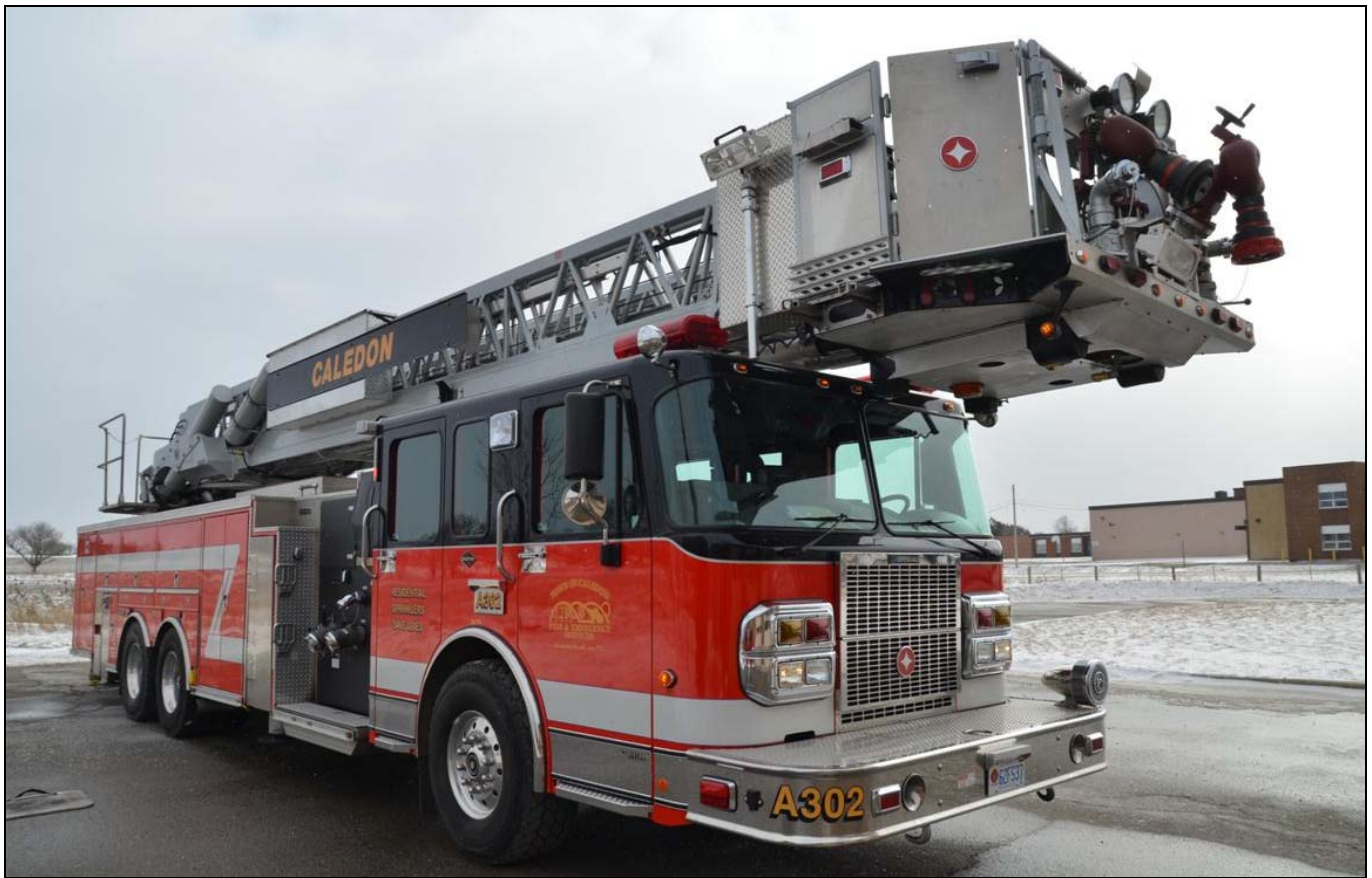
Another quint tower in service, belongs to Caledon and is currently being kept in Station 307 until larger accommodations are built in Bolton. The Crimson/DEV product was constructed on a Spartan Gladiator Classic chassis and was purchased from Dependable as a demo. (Larry Thorne photo)
